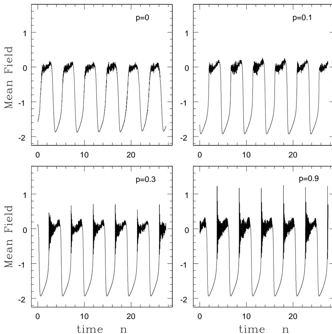
Figure 1: Time evolution of the collective field of networks of coupled Hindmarsh-Rose neurons, after a transience of  $10^4$ , with rewiring fraction  $p =$  (a) 0 (b) 0.1 (c) 0.3 and (d) 0.9. The system size is  $20 \times 20$ .
