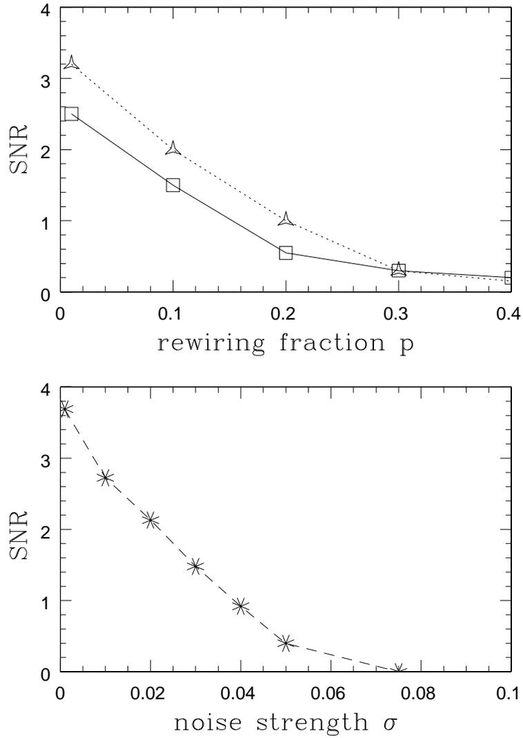
Figure 6: The upper panel displays the signal-to-noise ratio (SNR) of the power spectra of the collective field of coupled logistic maps for different values of rewiring fraction  $p$ . The lower panel displays the SNR of the power spectra for a regular network under different noise strengths  $\sigma$ . The system size is  $20 \times 20$ .
