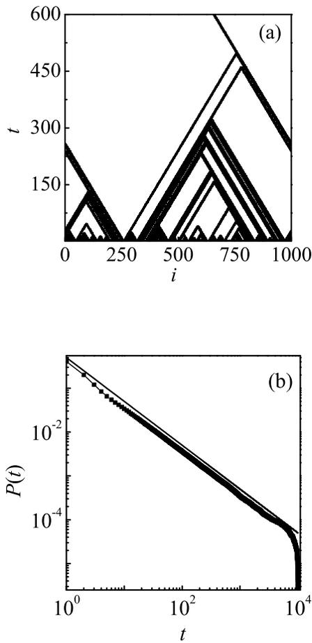
FIG. 3: (a) Representative spatiotemporal plot of the CA model. Sites with nonzero values are dark in this representation. (b)  $P(t)$  as a function of time  $t$  for the CA model, for  $N = 10^5$ . We average over 100 initial conditions. Clearly,  $P(t)$  goes as  $t^{-1}$ . A line  $1/2t$  is also plotted for reference.
